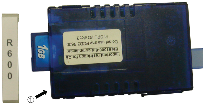
Fig.2-4 Installation of the SD Card into the Web Server Module PCD3.R600
